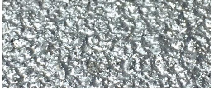
The guidelines shown below must be observed to insure that the galvanizing process does not damage SlipNOT® steel treated materials. SlipNOT® is not responsible for damage caused by third party operations such as galvanizing. *Note: Damage to the SlipNOT® surface is caused from over exposure to pickling acids.*
